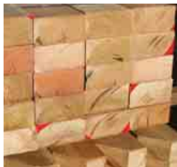
Picture shows sapwood (highlighted in red) in un-treated bollards
