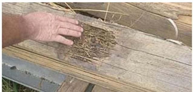
Area around vertical through bolt where Malthoid held water next to the wood bearer causing the cross bearers to decay in 8 years
