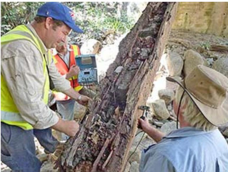
EPHOD (trademark) Electronic Pulse Highlight and Outline Diagnostic testing of failed stringer in Northern Queensland to establish the reading obtained in microseconds (ms) across a known defect.
