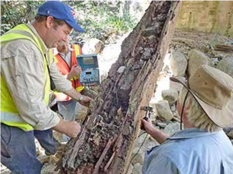
The annulus thickness at the point of bore sounding was over 100 mm. Clearly sounding bores are not satisfactory inspection methods for old timber bridges.
