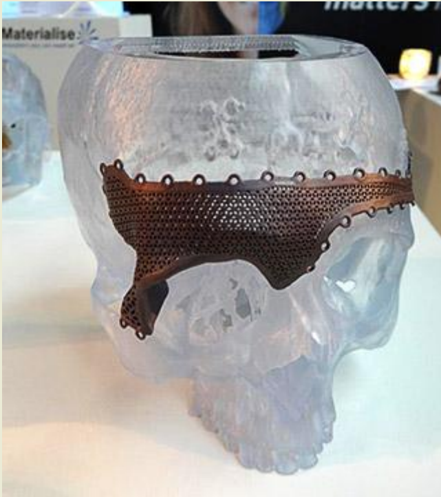
3D printed titanium plates for scanned face of patient with bone cancer
